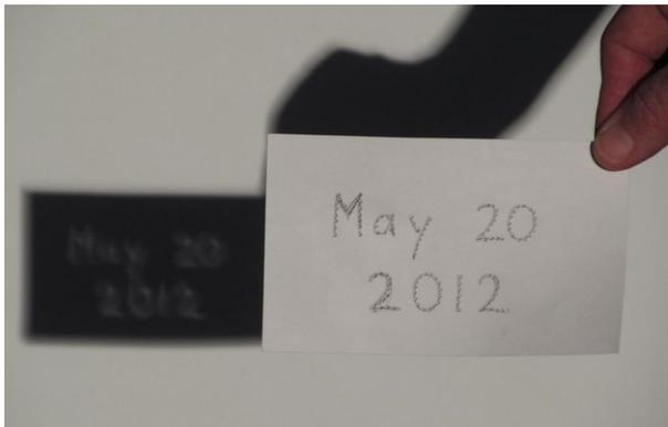
Pinhole shadows showing the date made with a pushpin and an index card.
