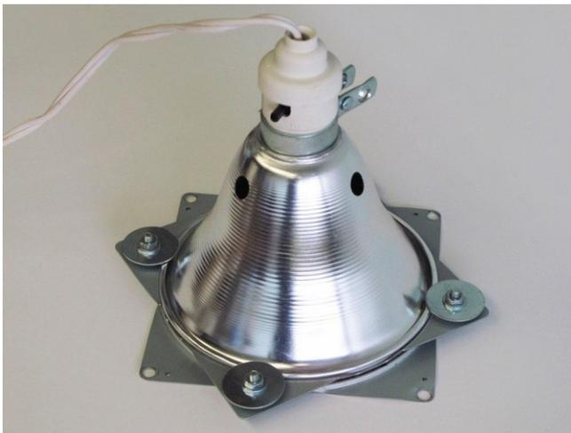
Add four long machine screw. On the side of the bearing with the holes near to the corners, insert a long machine screw into each corner of the bearing, pointing away from the lamp, and secure them each with a washer and nut.
